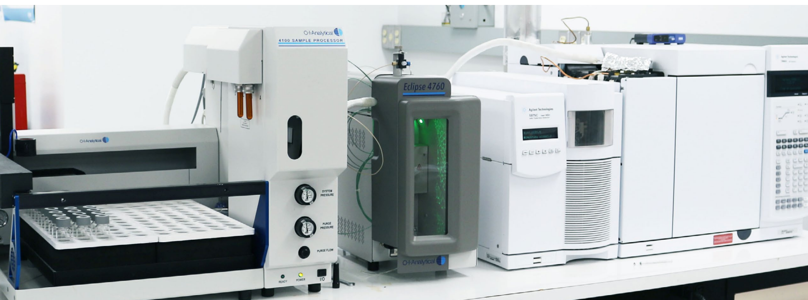
Figure 1. From left to right, the OIA 4100 Autosampler, OIA 4760 Eclipse Purge & Trap, and the GC/MS system.
